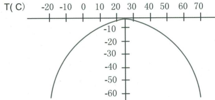
To determine frequency stability, use parabolic curvature
